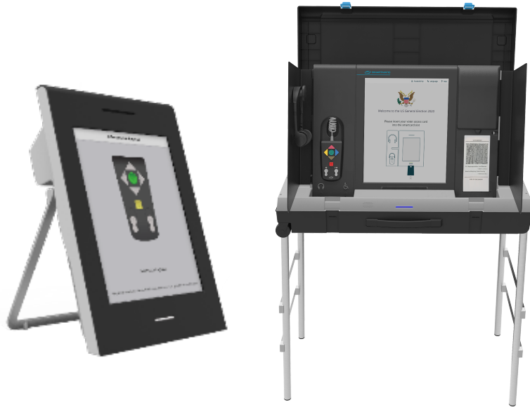
BMD with optional tabulation with C&D printer, or DRE with VVPAT 17" touchscreen voting machine
